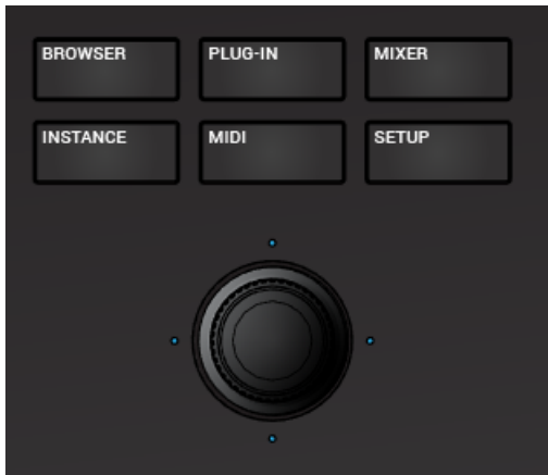
The 4-D encoder situated below the Mode buttons.
