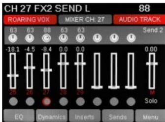
The Encoder group (P) to the right of the display is assigned by default to control EQ for the currently selected channel. Using the LED buttons (I) as Select buttons, you can select a new mixer channel without changing your current sequencer track. This is useful, say, if you want to tweak the EQ on a kick drum track while still playing a bass sound from the keyboard.
