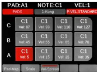
To change the velocity level for a pad, simply select it by tapping the pad and use the Data encoder (O) to change the value.
