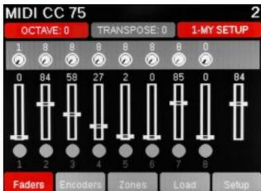
Move the faders and their values will update in the display as they move. Where controls are assigned to send a standard MIDI Controller message, pressing the **TOGGLE/VIEW** button (G) will display the Controller number assignments. Pressing the **TOGGLE/MUTE** button (J) will mute the MIDI output of the faders, so you can position them where you want them. Press again to unmute.
