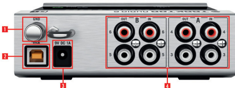
5.2 The rear panel of the TRAKTOR AUDIO 6.
