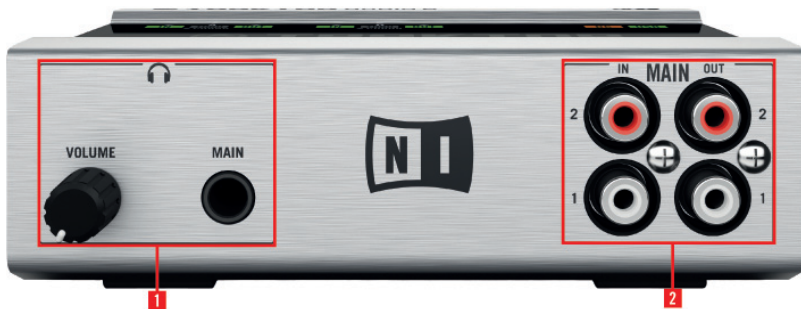
5.1 The front panel of the TRAKTOR AUDIO 6.
