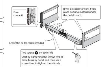
2. Holding the left and right side boards, raise them so that the pedal board 3 is not twisted.
