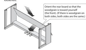
4. Use screws 7 to fasten the rear board 5 from the front to the metal brackets on the inside of the side boards.
